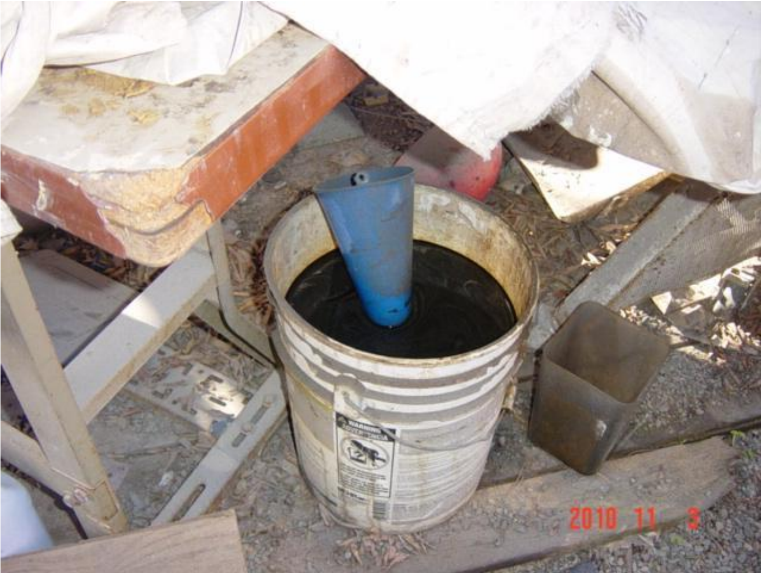
Open container of used oil observed near the hazardous waste storage area.
